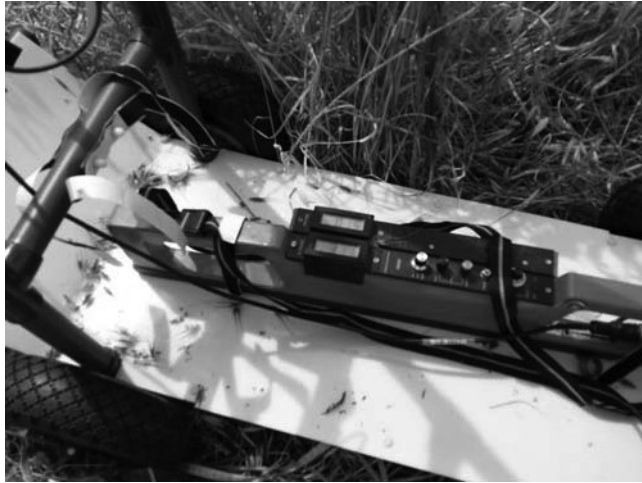
■ FIGURE 13.3 Electromagnetic induction instrument for the determination of bulk electrical conductivity (EM38, Geonics Limited).
